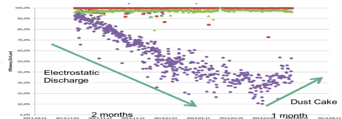
Figure 13: Efficiency trend data from mobile test laboratory
