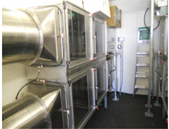
Figure 10: Mobile air filter test laboratory
